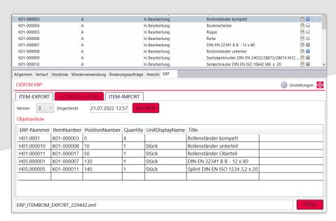
ERP information and integration functions are displayed on an additional tab in Vault Professional.
