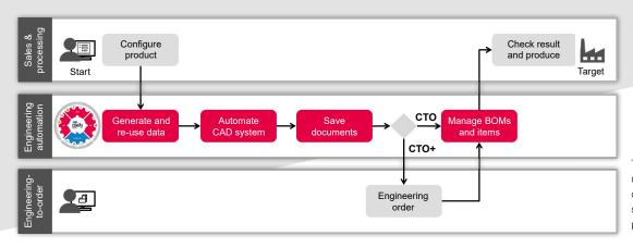
The configuration process using CIDEON Conify – from configuring products in sales through to transfer to production.
